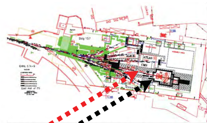
Figure: Beam lines in the PS East Hall. T7 and T8 are near the bottom. The maximum length is below 100 m.
