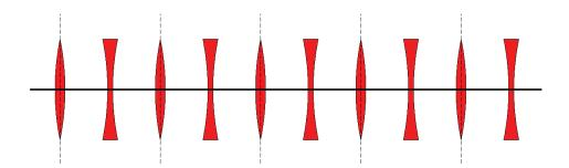
If we understand the dynamics in one cell of this beamline, we understand the optics in the entire beamline. Let's calculate the transfer matrix for a single cell.
