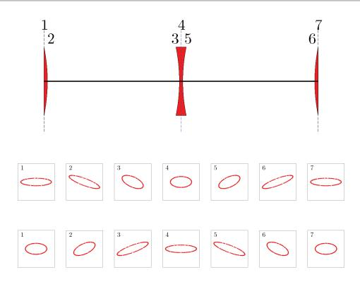
Horizontal (top) and vertical (bottom) phase space through a FODO cell.
