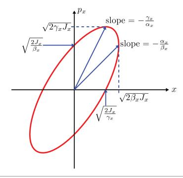
Consider a set of particles distributed around a phase space ellipse with a given action. As we move along the beamline, the shape of the phase space ellipse changes with the same periodicity as the beamline. At any given point in the beamline, the shape of the ellipse is given by the appropriate Twiss parameters.
