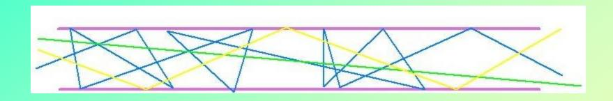
Particles are generated at random at the entrance and are followed through the system until they are either trapped (pumped) or exit at either end.
