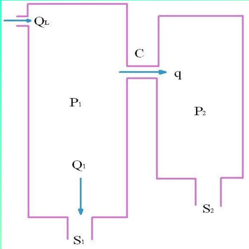
A common requirement is to maintain part of a system at a relatively low pressure while another part is at a relatively high pressure (e.g. an ion gun and a target chamber). We need to calculate the pumping speed  $S_2$  required to maintain the pressure  $P_2$
