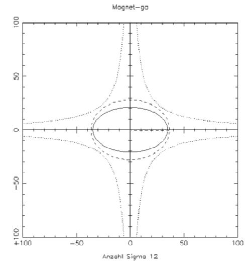
*typical beam envelope, vacuum chamber and pole shape in a foc. Quadrupole lens in HERA*
