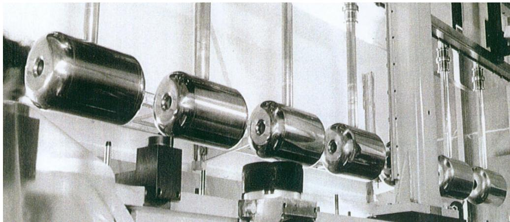
500 MHz cavities in an electron storage ring
