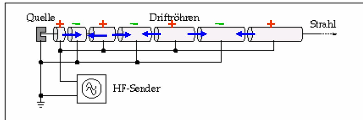
drift tube structure at a proton linac
