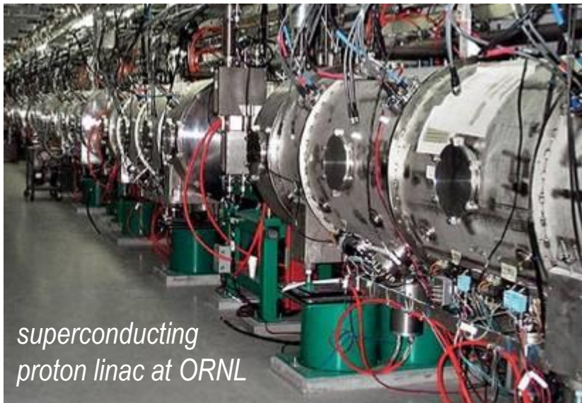
Superconducting Proton Accelerator 600 MeV - 2.5mA = 1.8MW
