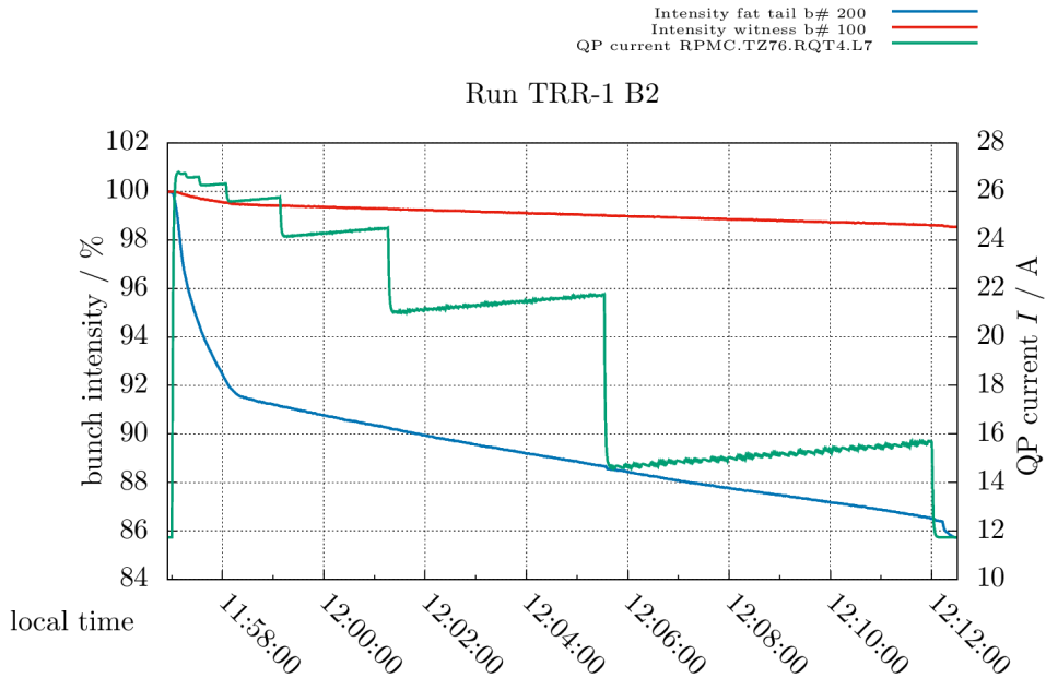
Figure 4: Nominal and fat tail bunch intensity in Beam 2 during the tune modulation. A clear intensity decrease in the fat tail bunch is observed while the nominal bunch intensity is slightly affected.
