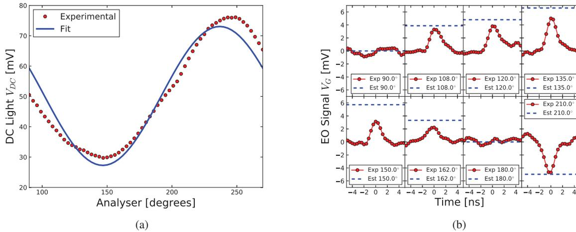
Figure 4: Analyser polarization scan of pick-up zero (a) and EO Signal for different analyser positions (b).
