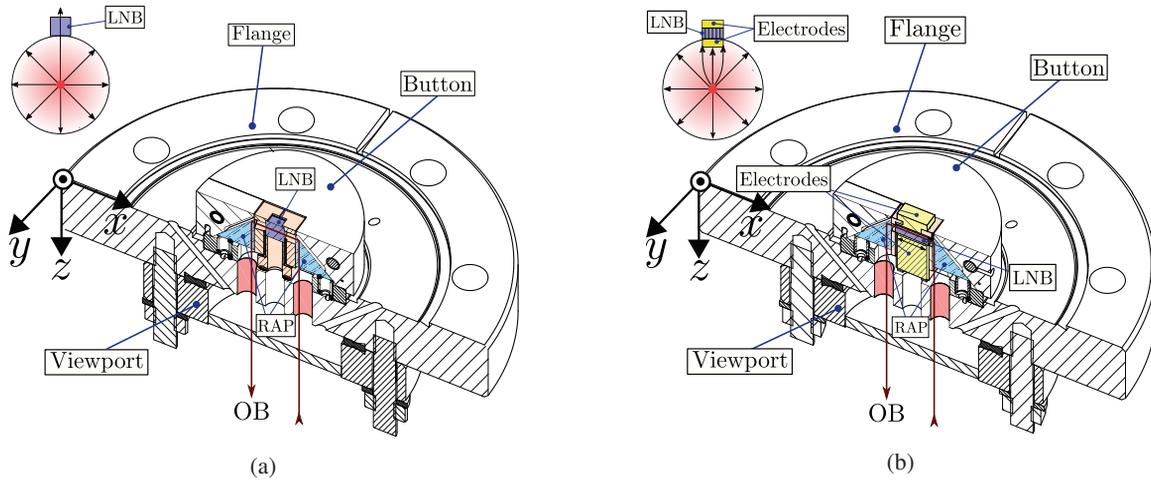
Figure 1: Prototypal pick-up variants: zero (a) with only a crystal; and one (b) with an additional electrode.
