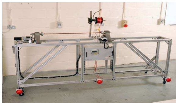
Figure 3: A test winding of 1-m long undulator prototype on a custom built winding g machine.
