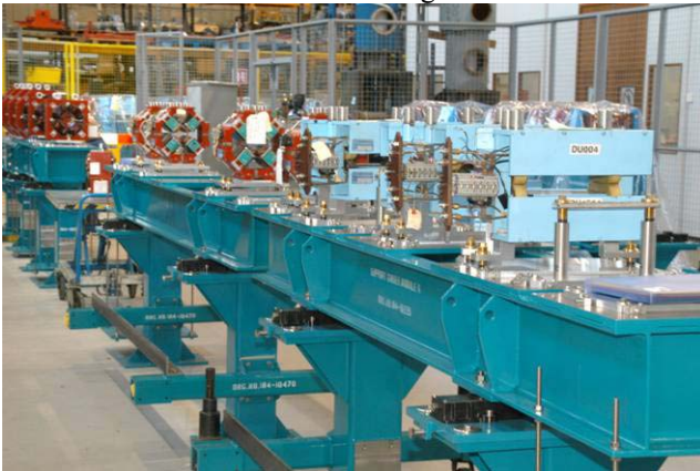
Figure 6: Modular girder assembly.
